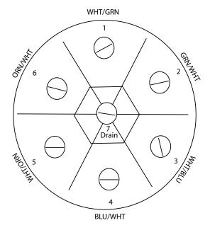
Figure 2-15 Wiring the socket insert
